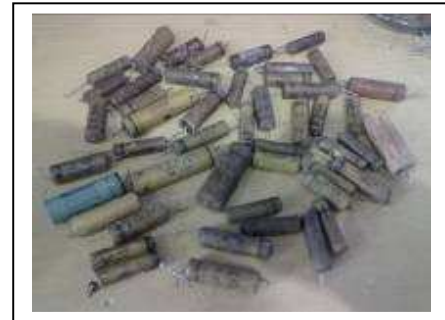
Old Capacitors removed from the receiver on the left
